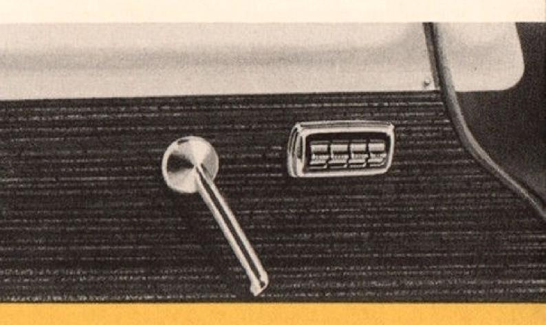
Master control switches are placed on the driver's door panel. There is also a switch under each window.
