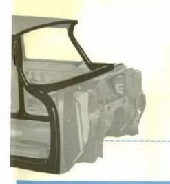
Herculite door glass—three times stronger than laminated glass! A Plymouth taxicab exclusive! Resists cracking or breaking no matter how hard and often the cab doors are slammed! Plymouth pioneered its use in taxi doors—to keep your cabs from layup time for broken glass replacement! A big saver of time and money!
