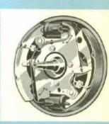
TOTAL CONTACT BRAKES, with new advanced step design—a Plymouth exclusive in the taxi field, are especially adapted to taxicab stop-and-go driving because the brake shoe follows the wheel drum as the drum expands from heat, maintaining safe stopping contact. Each front wheel has two brake eylinders. Stops are safer and surer, with 25% less pedal pressure. Plymouth brake linings are bonded to shoe... no rives to score drums.
