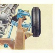
Torsion bars are one of the secrets of Plymouth's Torsion-Aire Ride. This famed suspension is standard equipment on every Plymouth built. You feel virtually no roll or sway on curves, even at speeds higher than you're likely to use in turns. You stay level taking corners, stop without dipping.
