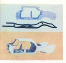
(Top) The way ordinary automobiles are made. A body unit is bolted to a frame unit. It is now going out of date.
