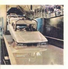
Raw steel just in from the mill is thoroughly scrubbed at 180° F. and protected before fabrication begins. Then, early in their manufacture, all new Plymouths are given seven different preparatory and protective baths and six chemical sprays which add extra years of wear to Plymouth's solid unit.
