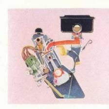
Plymouth's exclusive new 30-D Economy Six engine is inclined at a 30° angle. This saves space under the hood, and puts the carburetor, oil filter and other engine parts within easy reach for servicing. It also lowers the center of gravity and thus makes handling easier while also providing a much better ride.
