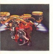
Manifold pipes 30 inches long act as sonic chargers. Some race track test cars, some hydroplanes use something like them. In Plymouth's importantly new SonoRamic Commando V-8 engine they ram far more torque into action for you than a conventional V-8. This engine is not for everyone. It costs extra.
