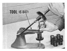
Use the valve spring tester (Tool C-647) next to see if compressed pressure and spring height at which you get the pressure are the same as that specified in the Service Manual. Any springs that do not measure up to specifications should be discarded.
