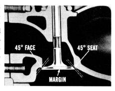
When you start your grind, feed the wheel slowly into the valve and take a very slight cut—not too much pressure. Next, feed the
