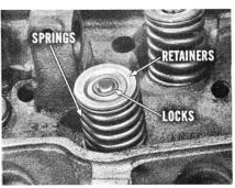
C-3648 to check the installed height of valves on all engines fitted with hydraulic tappets. Install new cup seals, too. Push them down into position over the end of the stem guides. If both the intake and exhaust valves had seals originally, replace *all* the seals with new ones. But if the engine you're servicing just had *intake* seals, replace only those.
