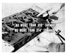
Gently move the valve head toward and away from the indicator. The total indicator movement should not exceed .010" on the intake or .014" on the exhaust valves. You'll have to ream the guides and install valves with oversize stems if the guides are worn.
