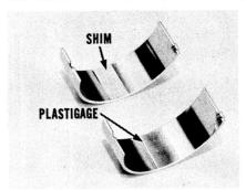
checking. In the first, you can use a small piece of oiled .002" brass shim stock, ½" x ¾" with smooth edges. Or, you can use the Plastigage method of measuring clearance. Whichever method you use, be sure to wipe the journal, cap and bearings clean first.
