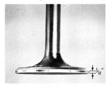
much and indicate that the valve had too much warpage to begin with. Too thin a margin can cause the valve to break or chip at the edges. What's more, the edges can overheat and cause pre-ignition or a popping back through the carburetor.
