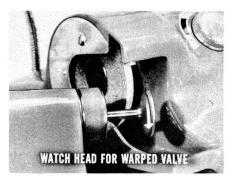
A valve slightly warped is serviceable if it can be refaced so that the margin is satisfactory. Margin is the unground edge of the valve. It extends from the top of the valve head to the upper limit of the face. What you're after is an angle of 45° on the face, and 45° on the seat.
