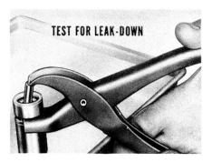
Hydraulic Tappets. If the engine has hydraulic tappets, you should remove the tappets for cleaning and inspection. Be sure to test all tappets for leak-down, and replace any that are not satisfactory.
