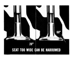
A seat too wide can be narrowed. Use a 20° stone on the upper surface, or a 60° stone on the lower surface. Location of the seat on the face will tell you which stone to use.
