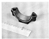
the cap and check width of the plastic against the graduated scale supplied with the Plastigage set. The scale reading will indicate the exact clearance. You can select the proper undersize bearing that will take up the clearance and leave the recommended .001" running clearance.
