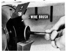
firmly against a wire brush mounted on a bench grinder. Clean the carbon off all surfaces . . . the valve head . . . the face . . . and the stem. Thorough cleaning is the important thing. If any carbon or gum remains, the valve might stick.
