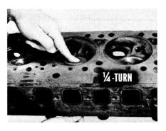
One good way to verify proper seating is to spread a thin coating of Prussian blue on the valve seat. Put the valve in the guide so the head rests on the seat. Turn the valve ½ turn, lift it up, and inspect the contact pattern. When possible, you want contact on the top of the face near the outer diameter of the valve.
