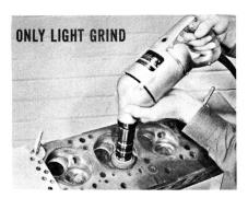
Reface the Seats. Truing up the valve seats is a precision operation. The seat must be square with the guide, and concentric within .002" total indicator reading. The angle of the seat must be the same as the face angle, 45° on V-8 engines.
