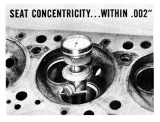
**NOTE:** If the seats are true, and were carefully ground, finish-grinding, or lapping in, isn't necessary.
